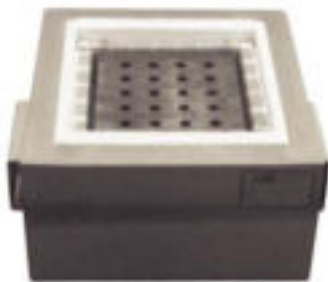
Special Series 3150 Box Furnace: Special construction with top lid assembly (not shown) and solid copper heat-equalizing block configured for simultaneous heating of 20 test tubes.
