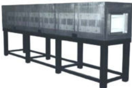
Series 3410 Multi-Zone Tube Furnace: Designed for continuous heat treatment of multiple strands of wire. Furnace featured 6 independently-controlled heat zones, each 24" (0.6m) long, for a total heated length of 144" (3.6m). Included a structural steel support frame.
