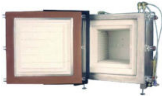
Series 3150CA Controlled-Atmosphere Box Furnace: Featuring water-cooled silicone rubber door gasket, cooling water manifold with control valves and flow sensor, gas ports, thermocouple ports, and vacuum pump, pressure regulator, and relief valve (not shown). See page 24 of this bulletin for more information.
